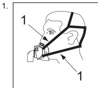
1. Gently pull each of the four side straps to achieve an overall even and balanced pressure and fit between the cushion and the face.
